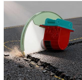
Diamond disc for cutting asphalt and concrete, compatible with mini, midi, and excavators from 1.5 to 6.0 tons. The standard disc is designed to work on a wide range of materials: bricks, granite, natural stone, porphyry, refractories, various types of concrete, and asphalt. If needed, or to adapt to different surfaces, it can be easily replaced with discs designed for other specific materials.
